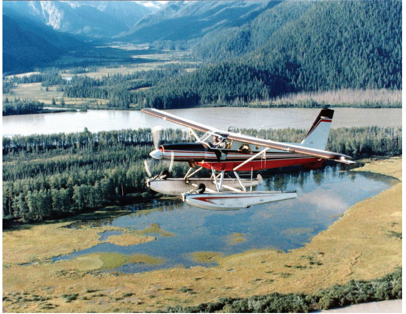
The Mk.III Turbo Beaver: an improved model developed in the 1960s with a Pratt & Whitney Canada PT6 turboprop engine
